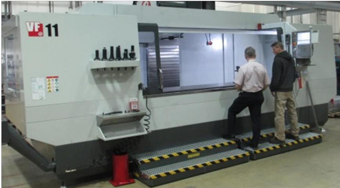
Five-Axis Hybrid AM Milling Center Working envelope: 120" × 40" × 30"
